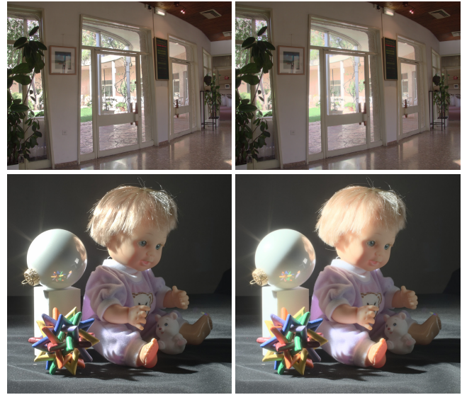
Figure 6: Our automatic mode results (left), compared to Reinhard’s global operator (right). The overall look is similar, but note the improved contrast in the brighter areas. (Doll HDR image courtesy of Yuanzhen Li.)
