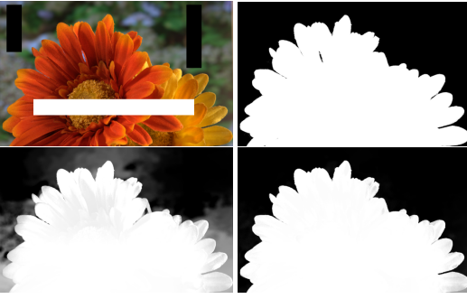
Figure 6: Closed form matting with diffusion distances. Top: input and ground truth. Bottom: corresponding results without (left) and with diffusion distances (right, t = 2 ).
