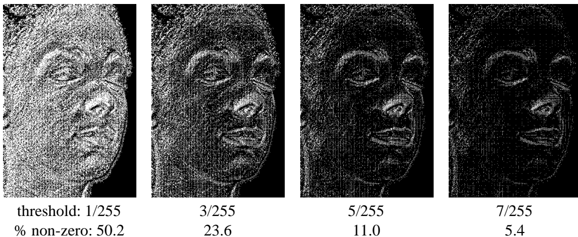
Figure 4: The wavelet-domain representation of the leftmost image of Figure 3. White pixels indicate non-zero wavelet coefficients. The leftmost image corresponds to a lossless wavelet transform. The remaining three images on the right show the result of lossy transforms, with the threshold increasing from left to right.
