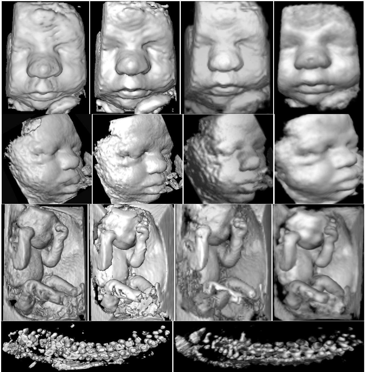
Figure 6: Rendering examples. The top row shows a fetal face rendered using ray-casting (left), Marching Cubes, shear-warp, and oriented splats (right). The second row shows another fetal face rendered using the same four methods. The third row shows a view of an entire fetus. The bottom row shows a spine rendered using Marching Cubes (left) and oriented splats (right).
